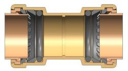
THE PROBITE<sup>™</sup> PUSH CONNECT TECHNOLOGY FOR PLUMBING, HEATING, AIR AND FLUIDS.
