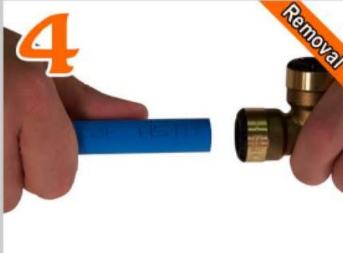
**Grip the fitting and the tube, pull the tubing from the fitting to remove. Once the fitting is released, remove the removal clip, then reassemble for reuse.**
