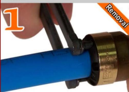
**With the system depressurized, loosen the retaining cap using the wrench and turn counter clockwise until the retaining cap is removed from the fitting.**
