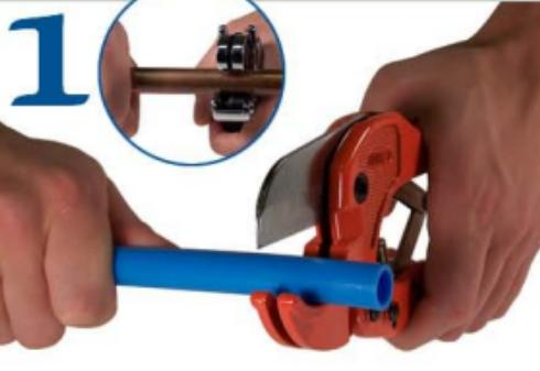
**Cut PEX, Copper, CPVC or SST tubing clean and square, removing burrs or sharp edges. Tubing should be round and free of score marks.**
