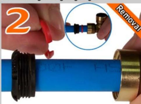
**Insert the removal clip by opening the clip and sliding it over the tubing with the sloped edge facing the inside of the fitting.**
