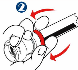
ProBite sealing O-rings (A) are easily removed and replaced (U.S. & Foreign Patents Pending).
